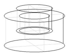
These kinds of intersections can be automatically detected by using the Geometry > Detect > Intersecting Volumes command. This function cycles through all the volumes in the model and tests for intersections with other volumes. Volumes that are found to intersect are highlighted as they are found for the user to review as below:
